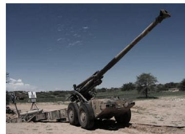
Fig 5: 155mm G5 Howitzer and precision munitions
